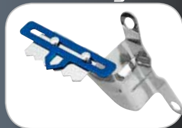
- Chrome Steel - 4241 - Big Blk Chev Adjustable 8" Balancer
