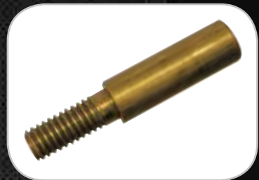
- Stud Extensions - 409-5993A - 50mm x 5/16" Unc 409-5994A - 86mm M8 to 5/16" Unc
